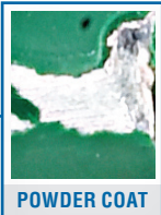
POLYURETHANE Crimped washer heads show polyurethane's superior durability while powder coating can chip and flake.
